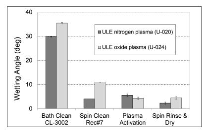
Figure 3: DI water wetting angles versus surface treatments for two ULE wafers
