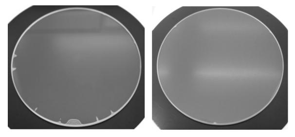
Figure 4: Bonded pair of SiO2 wafers (left) and bonded pair of ULE wafers (right)
