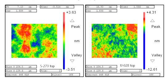
Figure 2: Surface roughnesses of a SiO2 wafer (left, ≈1.01 nm RMS) and an ULE wafer (right, ≈1.03 nm RMS)
