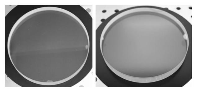
Figure 6: Glass wafer bonded to massive glass substrate of identical material (left: fused silica, right: ULE)
