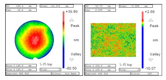
Figure 1: Surface flatness (left, ≈100 nm PV) and roughness (right, ≈0.4 nm RMS) of a massive SiO2 substrate
